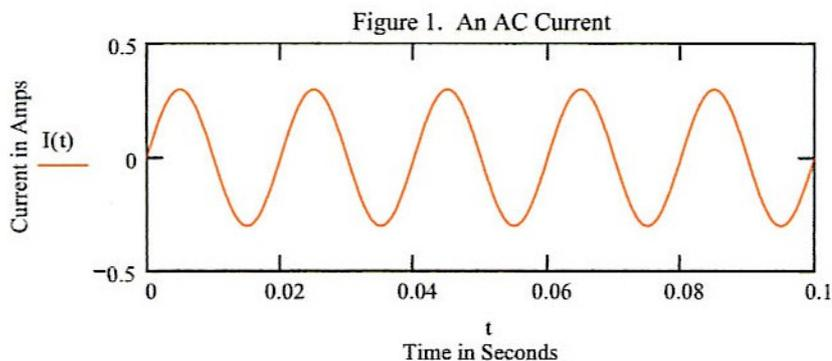
Common usage is to refer to a DC voltage or an AC voltage. The AC voltage will have the same shape as the current just illustrated but will of course have the units of Volts.
