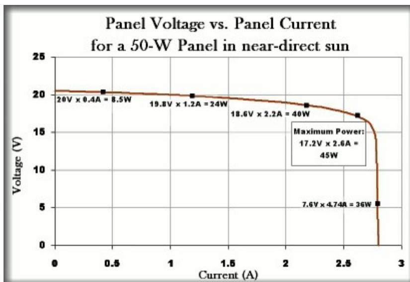
You can see that with no current taken out of it the panel will produce just over 20V DC. This will fall to about 17V when 2.5A is taken from it.
