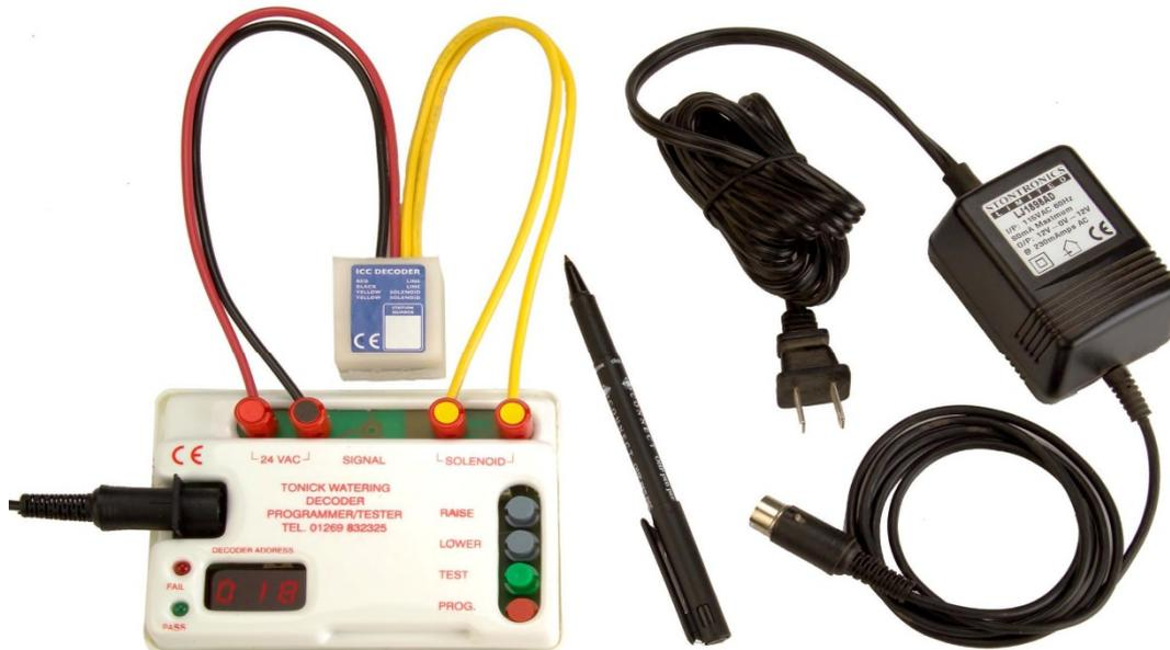
If one like this is not available, the controller itself can be used with the decoder wired directly into the 2 wire path terminals and a solenoid temporarily attached to give the decoder a load. Use Manual-single Station, set the required decoder number and then command the controller to Run.
