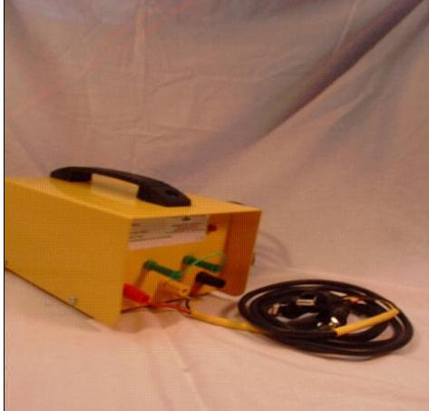
overheat. If at any time, faults are suspected, or the controller behaves erratically, it is best to test the wiring to the decoders using a power transformer and a current clamp meter.
