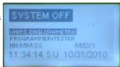
Scrolling down and pressing the ENTER/OK key will enter the decoder programmer tester screen. In this mode, decoders may be programmed with a station (zone) address, prior to installation onto the field wiring
