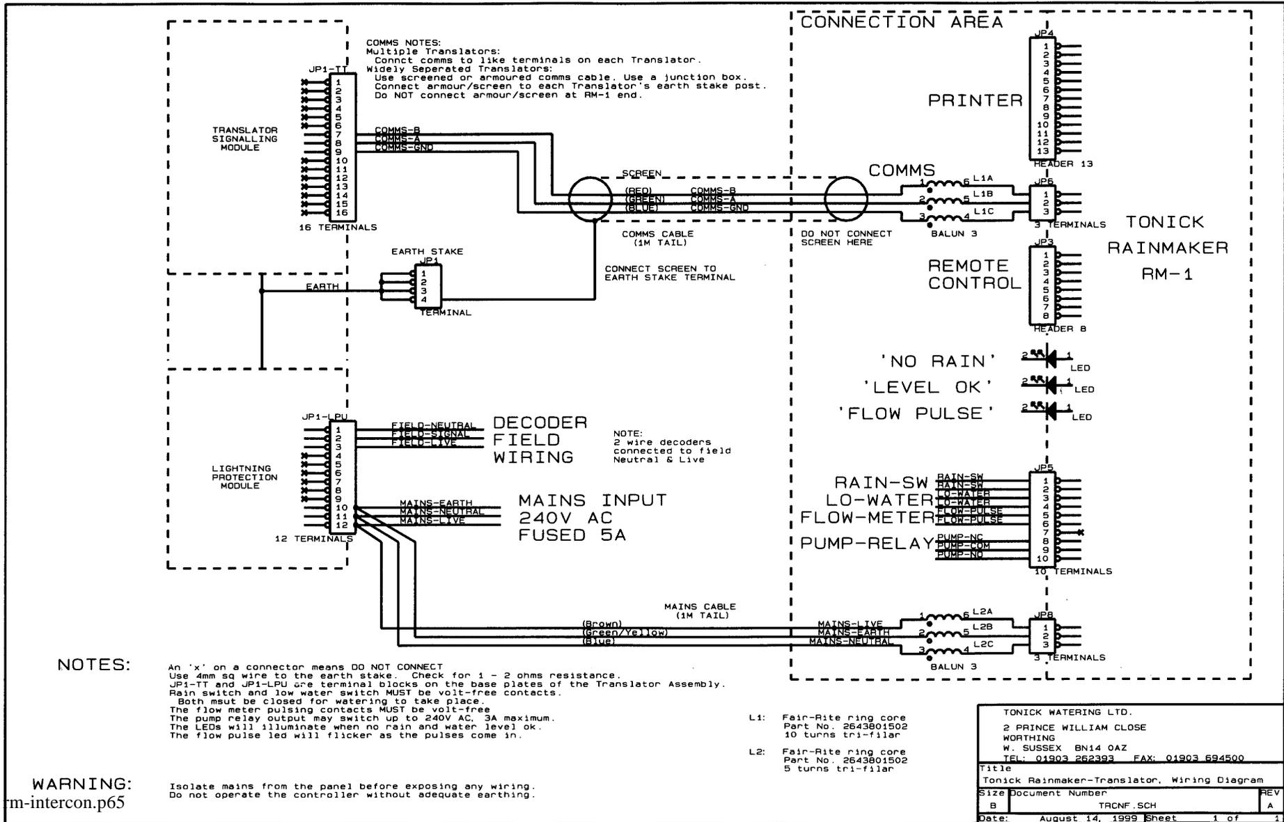
**Translators** translate general purpose station on/off commands from the RM-1 into the specific codes and signals to control a wide variety of existing decoder types currently in use. One Translator is used to energise each separate cable. Up to 4 can be connected to one RM-1
