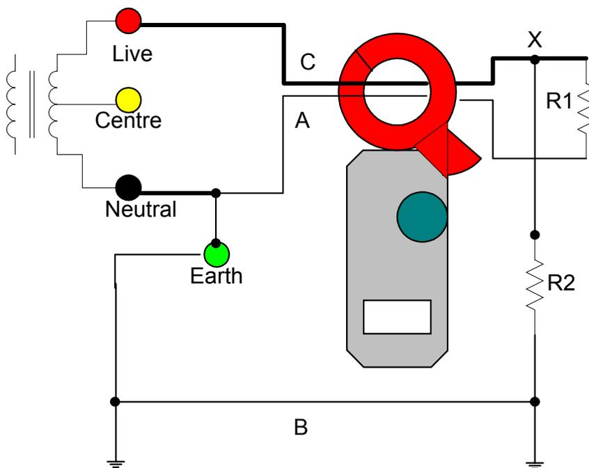
Contrast the previous diagram with that below. In this case the transformer is earthed on the same side as the leakage fault X. R2 instead of seeing the whole transformer voltage now only sees a small volt drop along the cable C. Therefore the current flowing in R2 is small and so the clamp meter reads almost zero.
