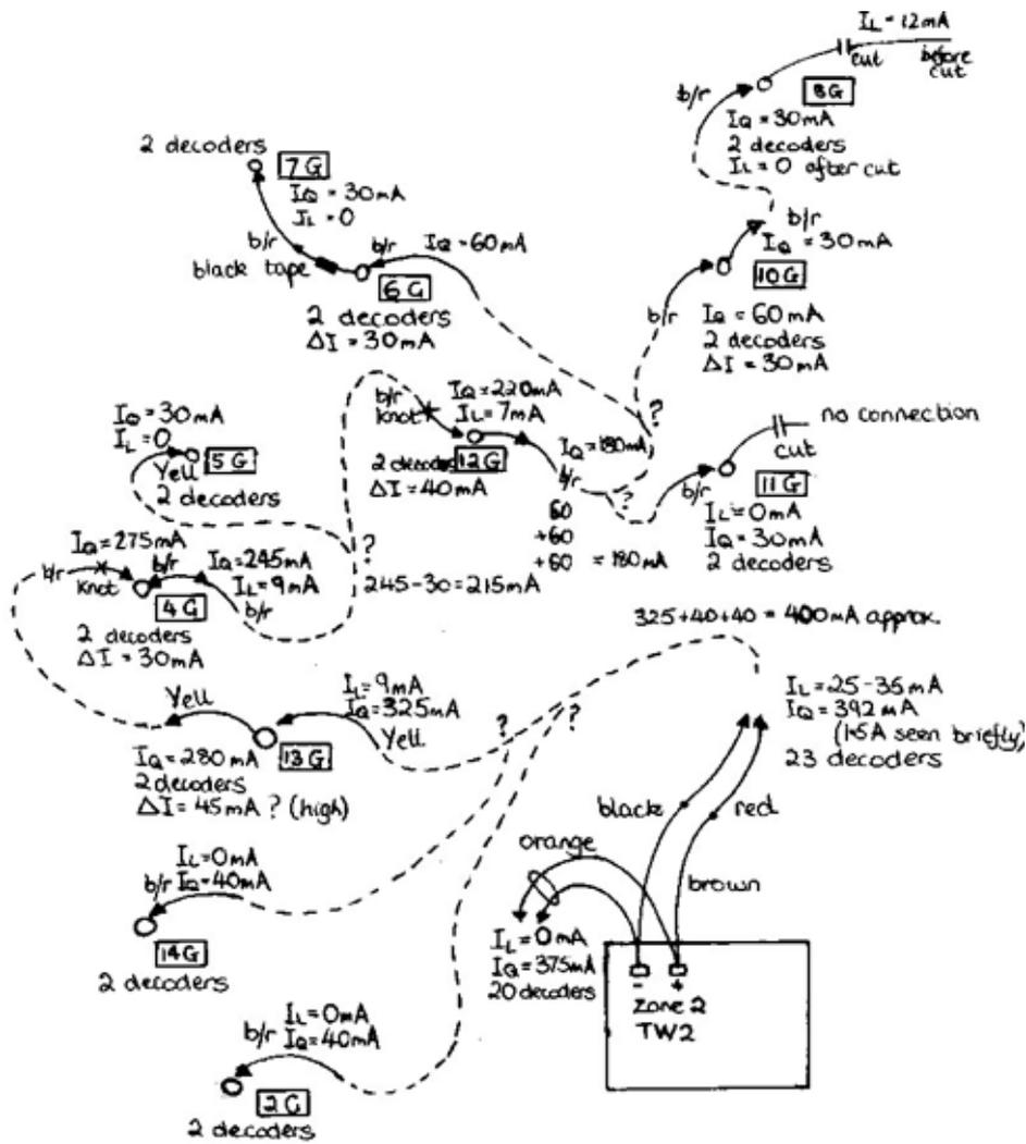
$I_L$  = Leakage current (mA) (after cutting the wire).
