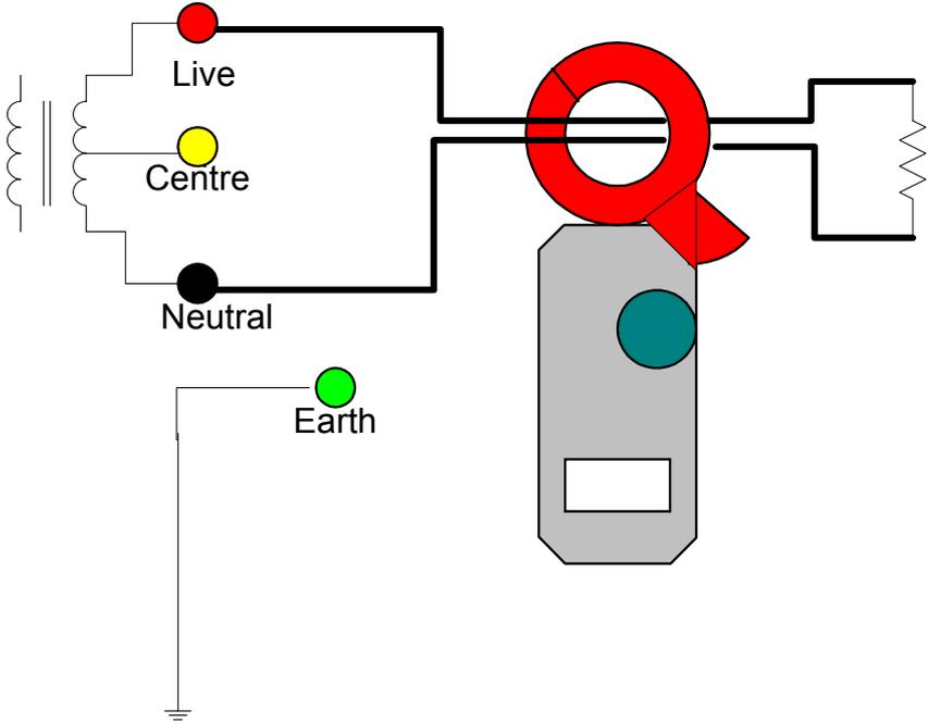
In the diagram below however, the current in C is returned partly in A and partly in B. The amounts apportioned according to the relative values of the two resistances R1 and R2. Because A and C are not equal, the current multimeter will read the difference (which is equal to that in B).
