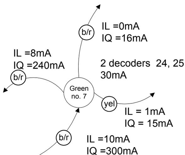
Having filled in the detail it is now necessary to join the boxes in the diagram. In the above example you would be looking for another box not too far away that has an incoming main feed of approximately 240mA and a leakage of about 8mA. Thus most of the boxes can be joined quite easily in an order of descending IQ.
