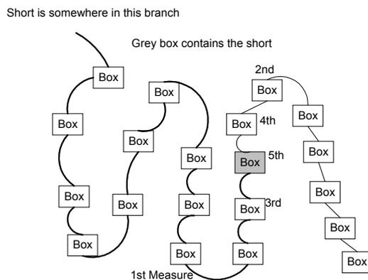
To measure the short circuit currents, place the current clamp over one of the power wires. On the other hand, if the short is between the signal and a power wire, place the current clamp over just the signal wire.
