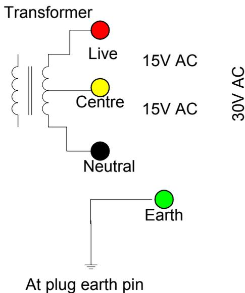
In the diagram the transformer's 240V primary is not shown.
