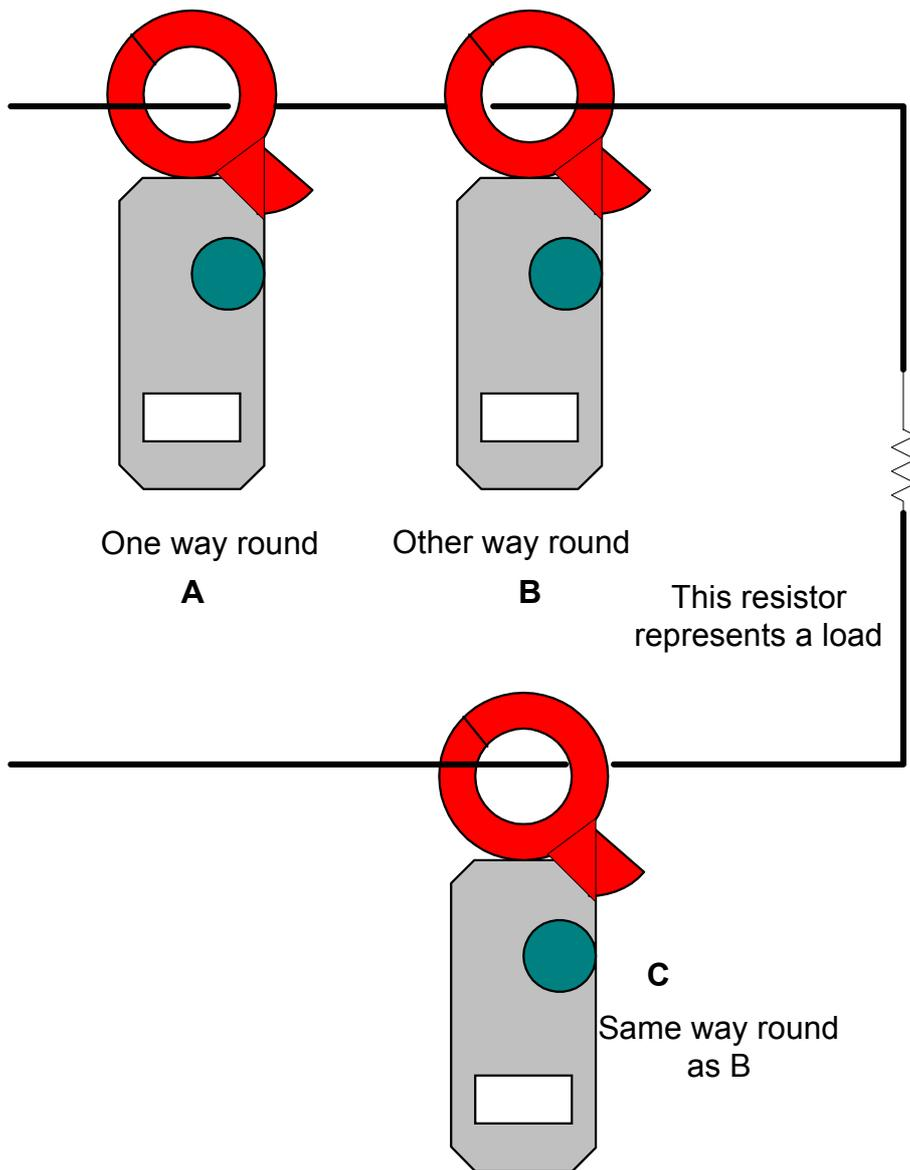
It is important to understand that if both flow and return wires carry the same current and are placed inside the jaws, *the multimeter will read zero* out.
