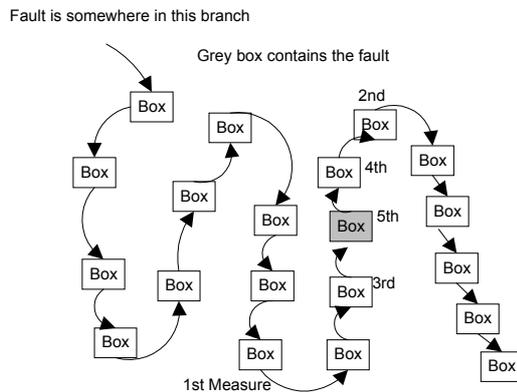
Measuring the standby currents down a run allows comparison between the number of decoders expected 'downstream' and the actual current. Most solenoids take 180-250mA so any excess current will show up much better if only a few decoders are 'downstream' rather than measuring at the transformer.
